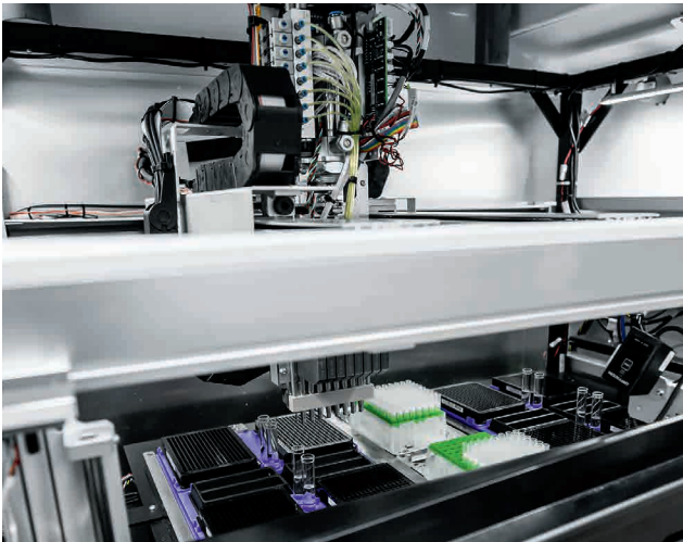
Maximum functionality in the smallest installation space: the planar surface gantry EXCM-30 is perfect for use in laboratory processes such as the dosing application shown here.
